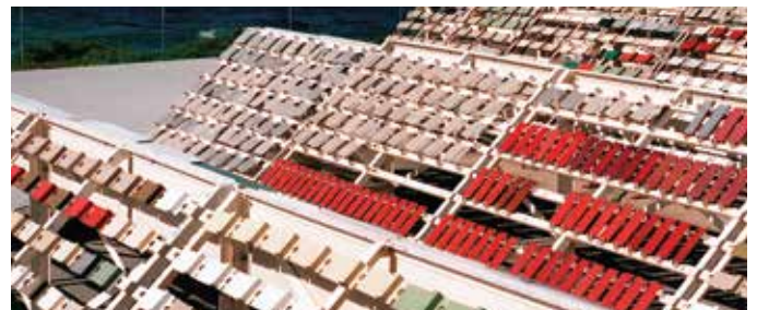
Figure 2: Test panels placed at BlueScope exposure rack
