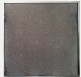
ZINCALUME® steel (No Sign of Rust)
