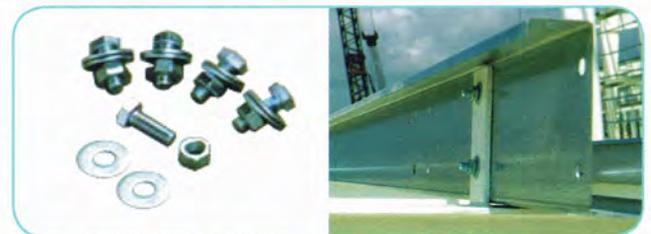
LYSAGHT purlin bolts and nuts have integral washers. Tighten all bolts to 55 Nm torque.
