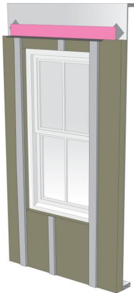
Step 16: Adhesive membrane strip extends past cap flashing.
