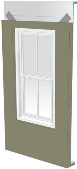
Step 13: Install ROXUL COMFORTBOARD IS insulation.
