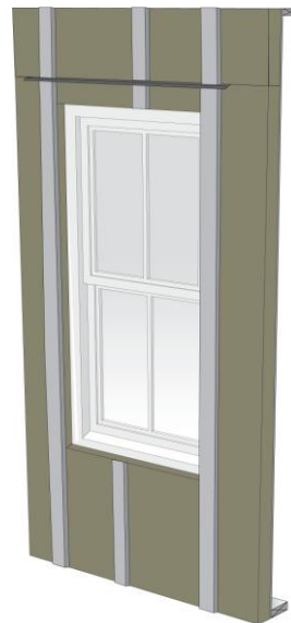
Step 18: Install next course of ROXUL COMFORTBOARD IS and furring. Drainage gap created by furring. Do not fasten furring through head cap flashing.
