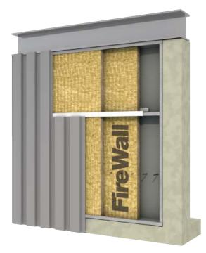
Components: Exterior Metal Cladding, Roxul FireWall®, Z-Bar Grits, Ceramic Fire Blanket (Z-Girt Cover), Flashing Channels, Wall and Partition Facings/Accessories
