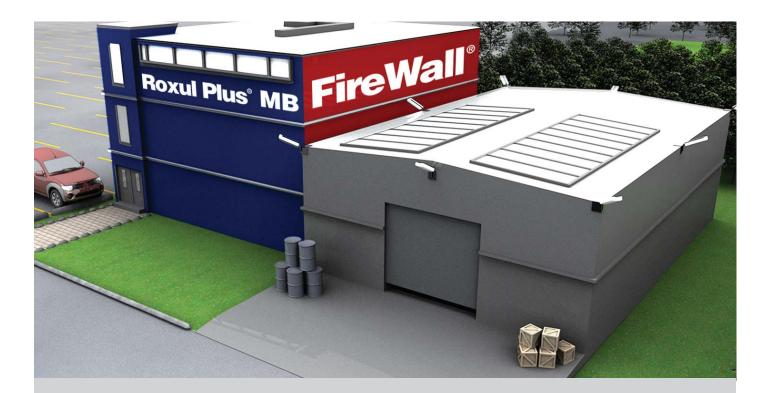
Roxul FireWall<sup>®</sup> and Roxul Plus<sup>®</sup> MB products are used to insulate walls in pre-engineered metal buildings. Roxul FireWall is ideally suited for zero lot line applications where buildings are in close proximity and fire safety is essential.
