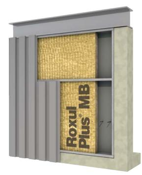
Components: Exterior Metal Cladding, Roxul Plus® MB, Z-Bar Girts, Flashing Channels, Wal and Partition Facings/Accessories
