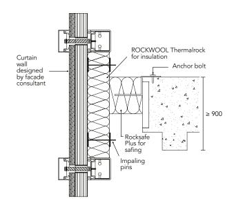
Sectional view of Rocksafe at perimeter edge of curtain wall
