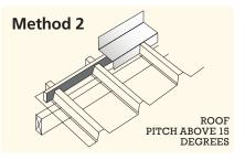
Where roof installations require Topglass<sup>®</sup> or Topclad<sup>™</sup> to be laid side-by-side, it is recommended that the use of Lap Seal Tape be implemented in these situations, therefore preventing possible water ingress over the laps.
