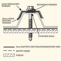
Inserted under the load spreading washer will be a 36mm EPDM sealing washer which is to be correctly seated to provide an effective seal. Fasteners should be inserted through the top centre of the rib/corrugation.
