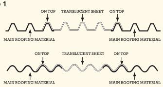
roofing profile will meet the spanning requirements. Contact Alsynite One NZ Ltd for specific design advice or refer Load Span Capability Chart -Page 24.
