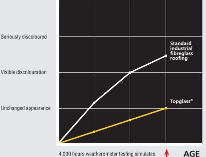
4,000 hours weatherometer testing simulates 10 years exposure in normal conditions
